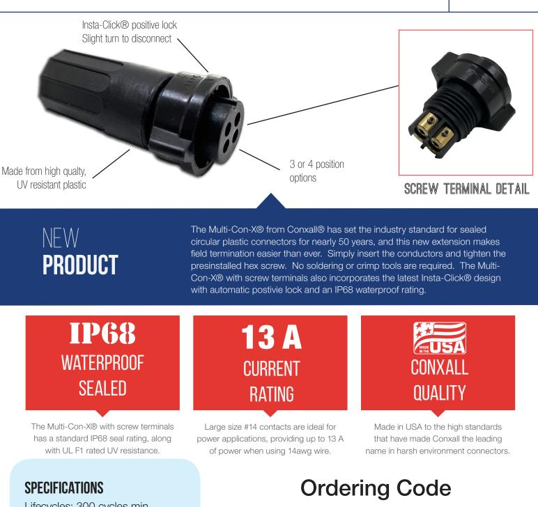
Lifecycles: 300 cycles min. Contact Size: #14 contacts Wire Size: 14, 16, or 18awg Voltage: 600V AC/DC Temperature: -40°C to 115°C Contacts: Gold plated copper alloy See drawing for additional specs.
